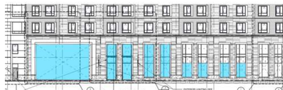
Figure 4 – Exterior wall openings
